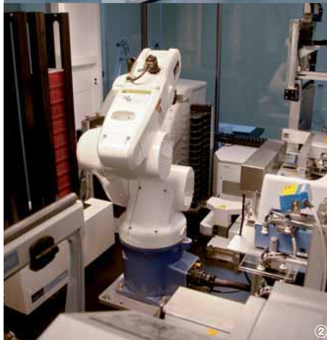
Assay automation: 1) 384-Well plates containing host cells infected with parasites are loaded onto an automated platform for compound addition, incubation, and reading. 2) Robotic arm involved in the process (High-throughput screening at Institut Pasteur Korea).
